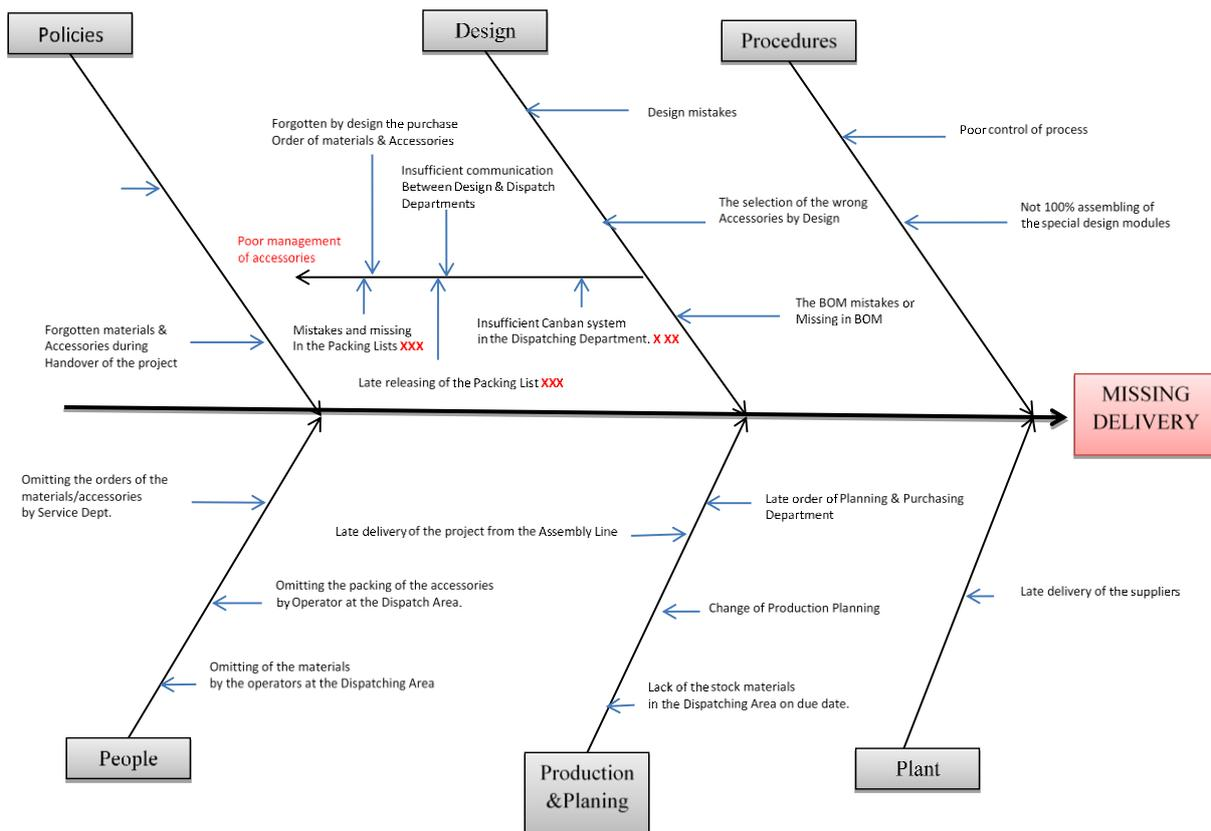
Figure 4. Cause-and-Effect Diagram
