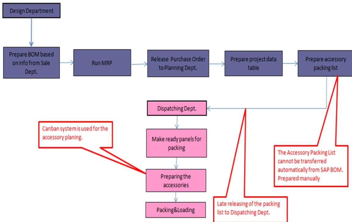
Figure 3. Process Flow Chart for Missing Delivery Issue
